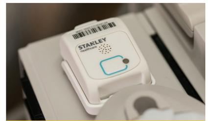
Wireless, battery-powered RTLS tags are available in varied form factors & functions
