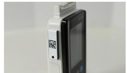
RAIN RFID (passive) tags are ideal for tagging smaller, mobile assets
