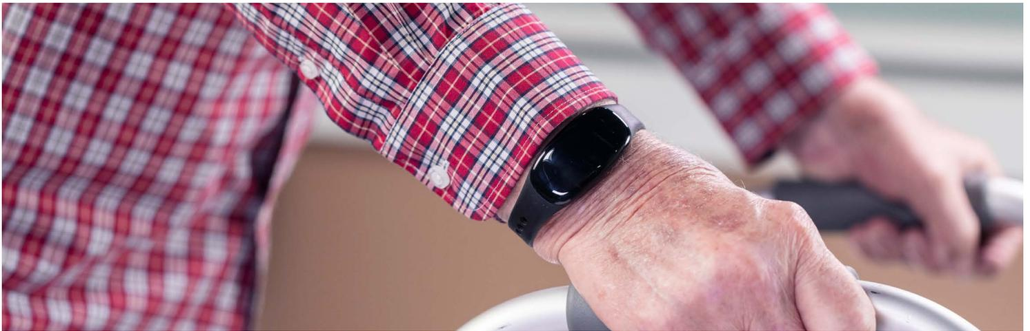
For example, when a supervised device is detected outside of its area, an “Out of Area” alarm can be generated by Arial and sent to caregivers so they can find the resident and bring them back to their normal area in the building. An “Out of Range” alarm occurs when the supervised device is no longer detected. The alarms clear when residents return to their assigned area.
